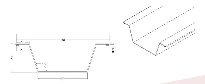
All of our metal profiles are manufactured in compliance with ASTM 635C and materials used in production comply with ASTM C955-11A. In addition, our standard sheet metal thickness is 0.6 mm with 120 gm/m² galvanization and 3000 mm in length. In addition, we have the capability to produce different thicknesses from 0.4 up to 1 mm, galvanization up to 275 gm/m², and lengths up to 6000 mm.
